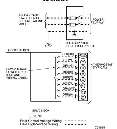
Fig. 5—50JZ High- and Control-Voltage Connections
